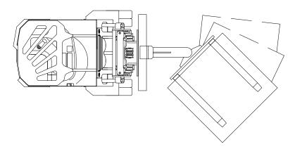
w DO NOT rotate the turret attachment when loaded unless the load is in a lowered position. This could cause the truck to tip.
