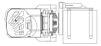
**w** Travel with the load in a lowered and centered position. This will increase the truck stability and operator visibility.
