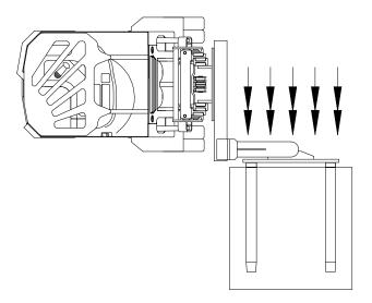
w DO NOT sideshift the attachment when loaded unless the truck is in a storage rack area or in a lowered position. This could cause the truck to tip.
